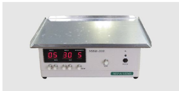
Figure 1. The NSB-100 device (Naga Co., Ichikawa, Chiba, Japan) used for the mechanical agitation of the in vitro culture system. Petri dishes contain the fertilized oocytes, and embryos are placed in the machine's CO 2 incubator. Scale bar = 5 cm.
